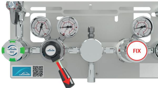
By turning the lever of the left pressure regulator anti clockwise all the way to the stop, the outlet pressure of the right pressure regulator is higher (approx. 2 bar) than the outlet pressure of left pressure regulator. As a result the manifold starts with taking gas from the right side.
